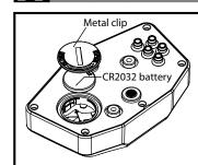
T After open the battery cover. please use the slotted-head screwdriver to take the battery
