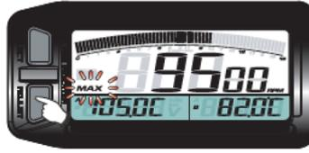
● MAX record screen, press the Adjust button once to go back to the sensor A screen.
