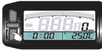
● In the sensor A screen, press the Adjust button once to enter the sensor B screen.
