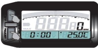
● In main screen, press down the Adjust+Select buttons at the same time for 3 seconds to enter the setting screen. (Check section 4-3 for detail)
