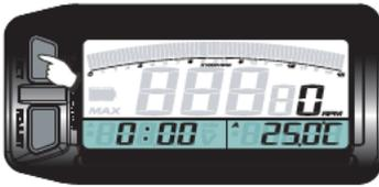
● In the clock screen, press the Select button one time to enter into the volt screen.
