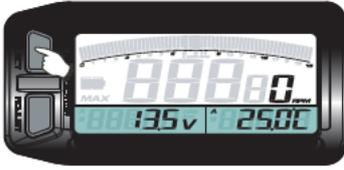
● In the volt screen, press the Select button once to enter into the sensor A screen.
