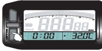
● In the sensor B screen, press the Adjust button once to enter in the Max. record screen.
