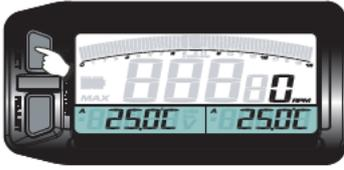
● In the sensor A screen, press the Select button once to enter the sensor B screen.
