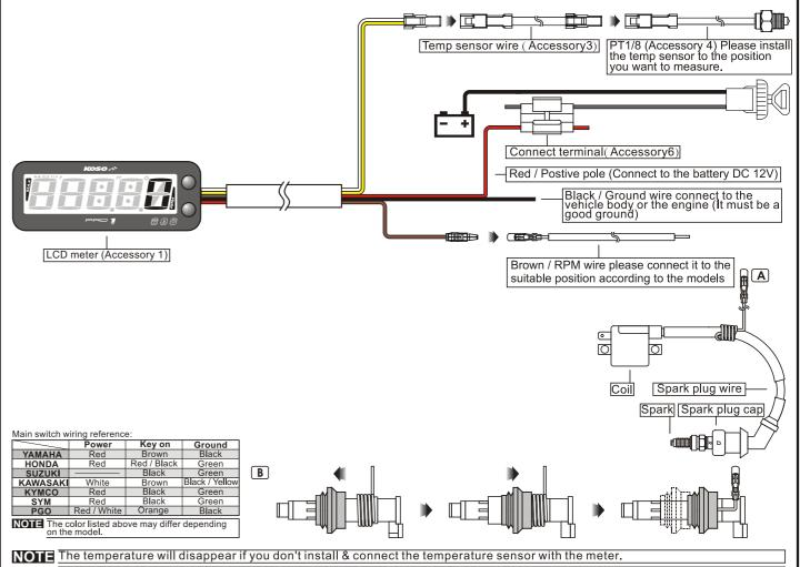
When connecting the power wiring, please follow the instruction. If you connect the brown wiring in parallel will cause the meter
