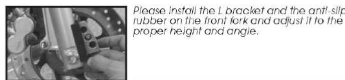
Please install the L bracket and the anti-slip rubber on the front fork and adjust it to the proper height and angle.
