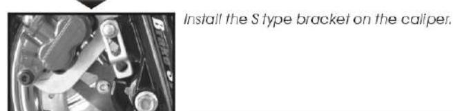
Install the S type bracket on the caliper.
