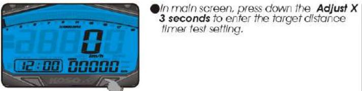
In main screen, press down the **Adjust X 3 seconds** to enter the target distance timer test setting.
