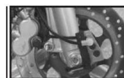
Please install the speed sensor into the proper hole on the bracket.
