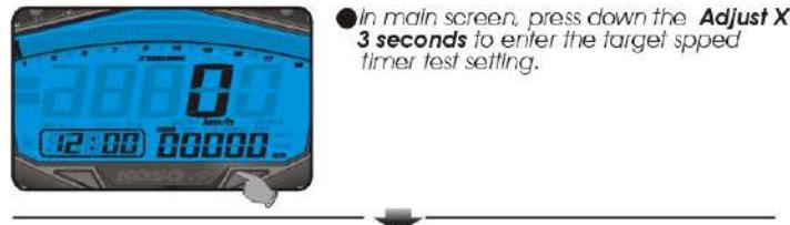
In main screen, press down the **Adjust X 3 seconds** to enter the target speed timer test setting.
