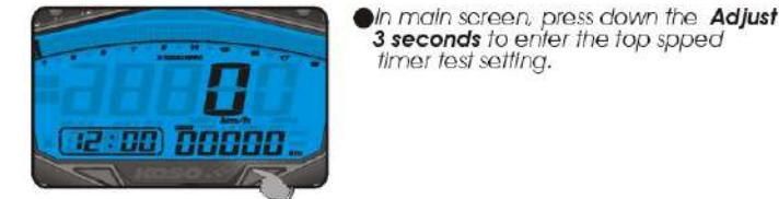
In main screen, press down the **Adjust X 3 seconds** to enter the top speed timer test setting.
